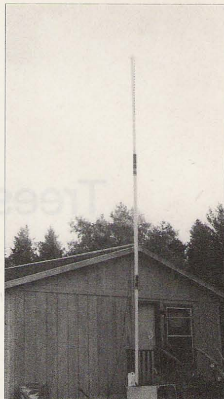
Photo C. The three-inch by 30-foot mast at work.
